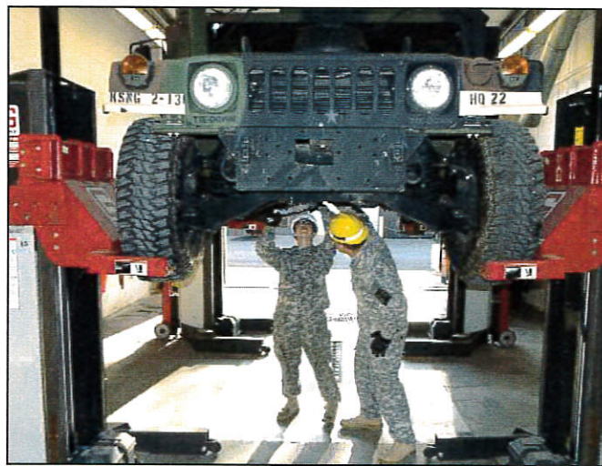
CSMS employees Sgt. Sherokee Knight and Spc. Lucas Greer tighten starter bolts with a torque wrench after replacing the starter on an 1165A1 HMMWV.
