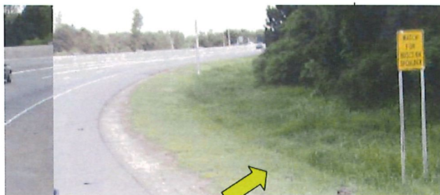
Watch for Buses on Shoulder sign (posted at entrance ramps or cross streets)
