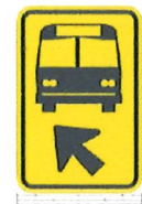
Exception sign (posted at "pinch point" on BOS)
