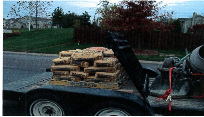
Numerous Load Securement Issues
