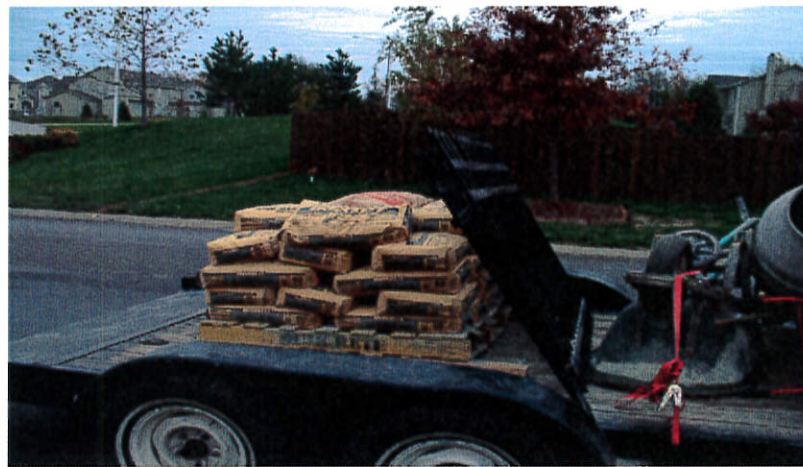
Numerous Load Securement Issues
