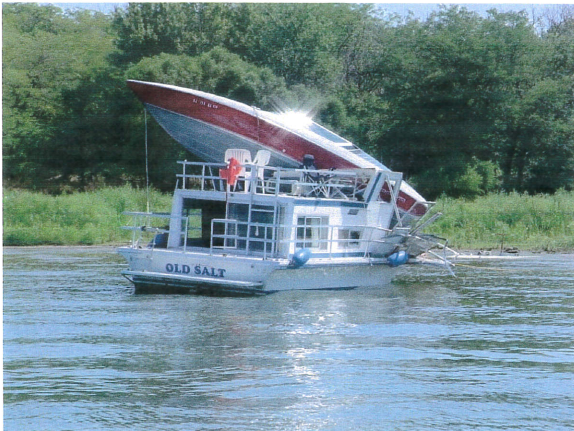
PERRY RESERVOIR – AUGUST 2003 IMPROPER LOOKOUT; IMPROPER LIGHTS; FAILURE TO HEED THE RIGHT OF WAY
