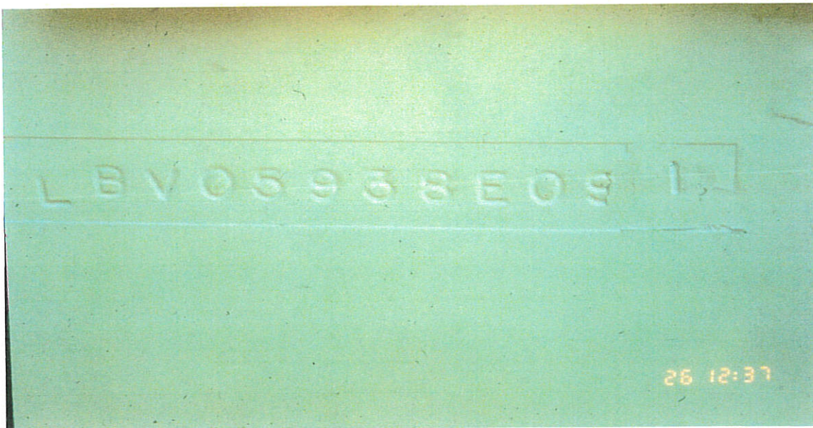
Stolen boat. Hull Identification Number that used body putty to change the last number.
