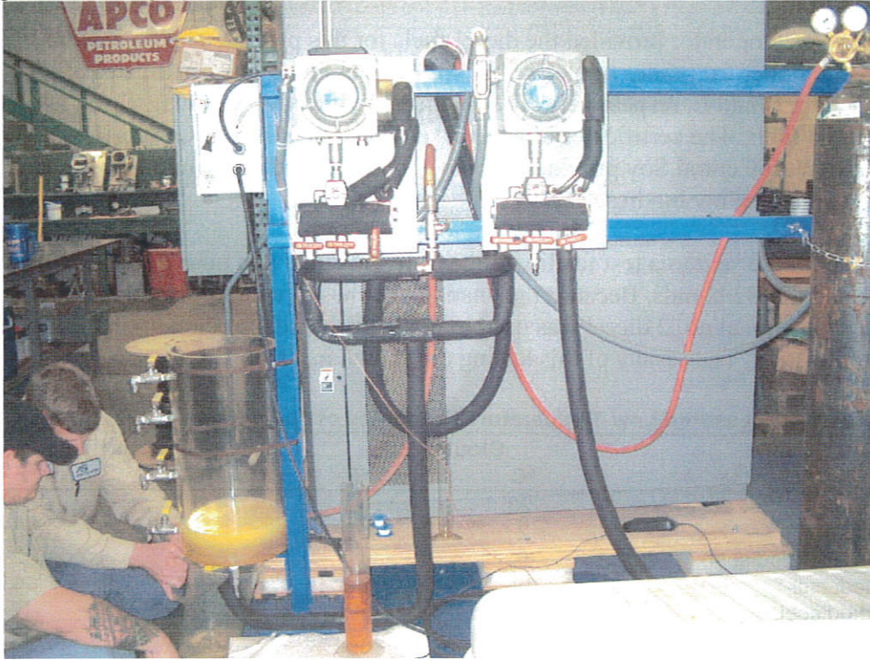
Figure 1. Photograph of Small Scale Test Unit for Blending Biodiesel and Diesel Fuel
