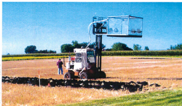
USDA scientists use this custom-built machine to study the impact of various tillage practices on soil carbon.
