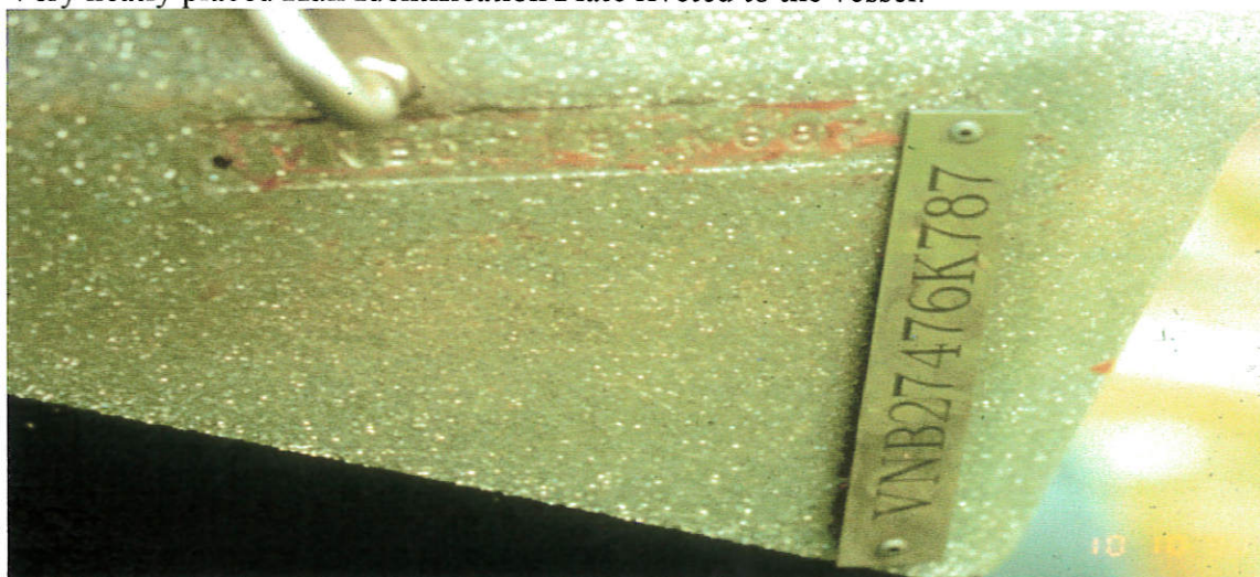
Same plate removed reveals original HIN stamped into the hull of the vessel.
