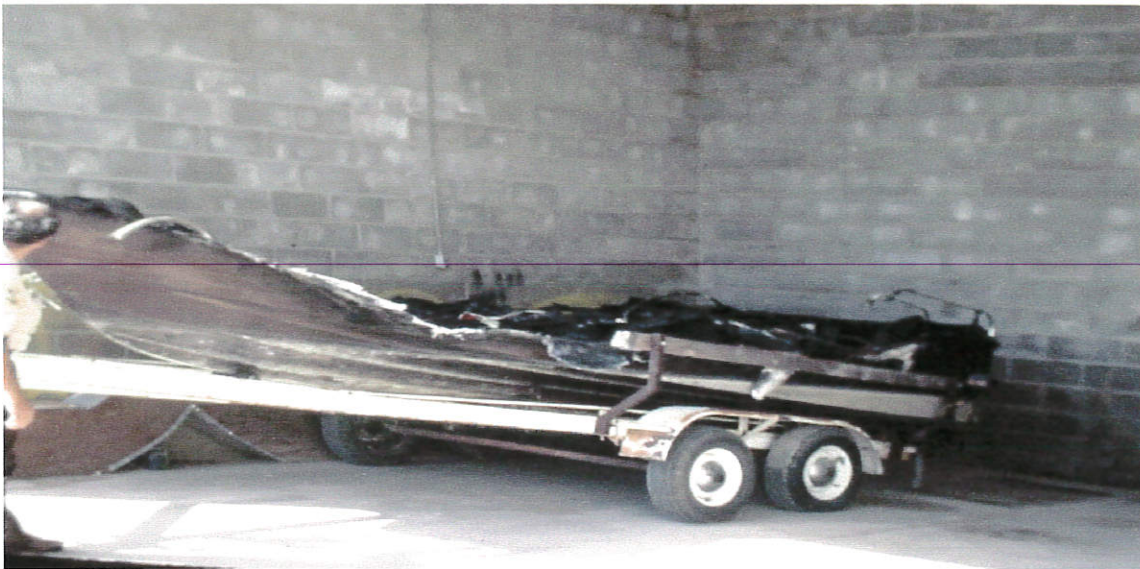
Vessels such as this burned vessel, which may only be identified by the HIN that remained on the back of the vessel. Heat from the fire melted the registration numbers.
