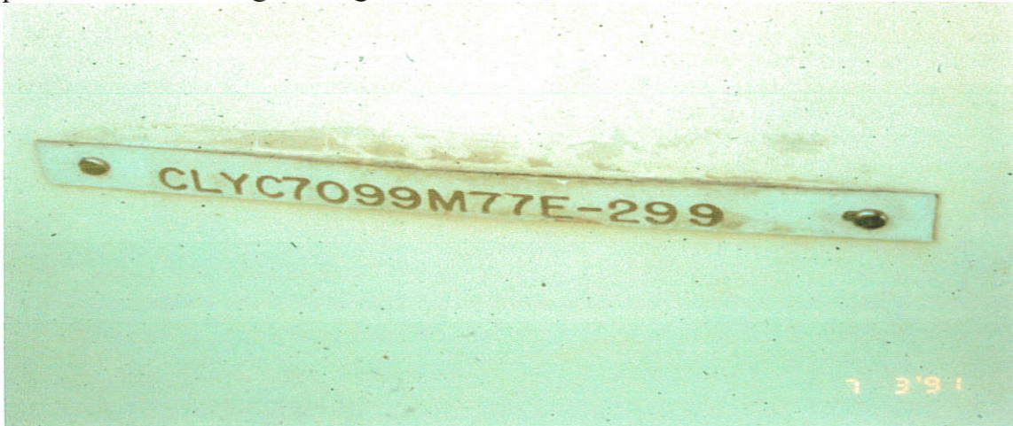
Hull Identification Number on a plate screwed to the hull of the vessel.
