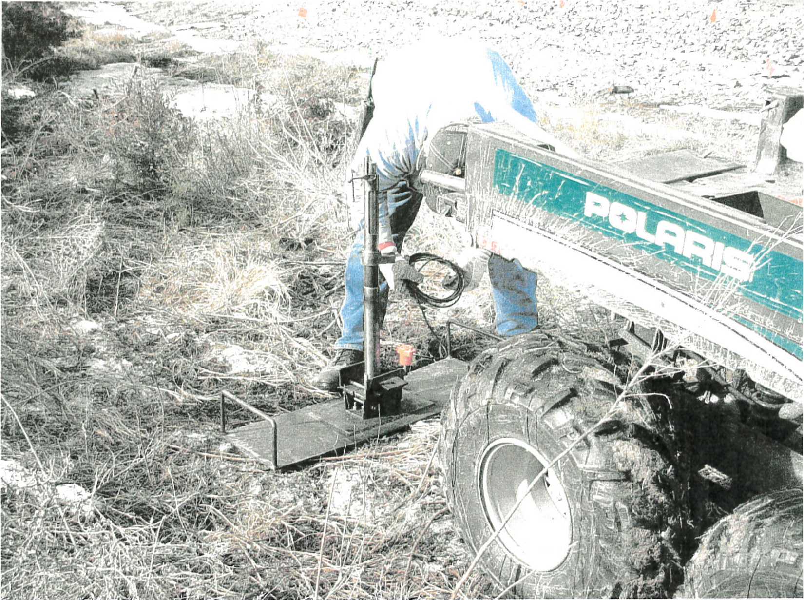
Kansas Geological Survey 50 Caliber Shot Seismic Energy Source
