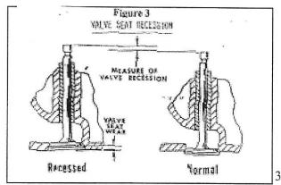
deposits on exhaust valve seats. These lead oxides prevented metal to metal contact between the exhaust valve and exhaust valve seat thereby preventing exhaust valve seat recession (EVSR) in engines without hardened valve seats.
