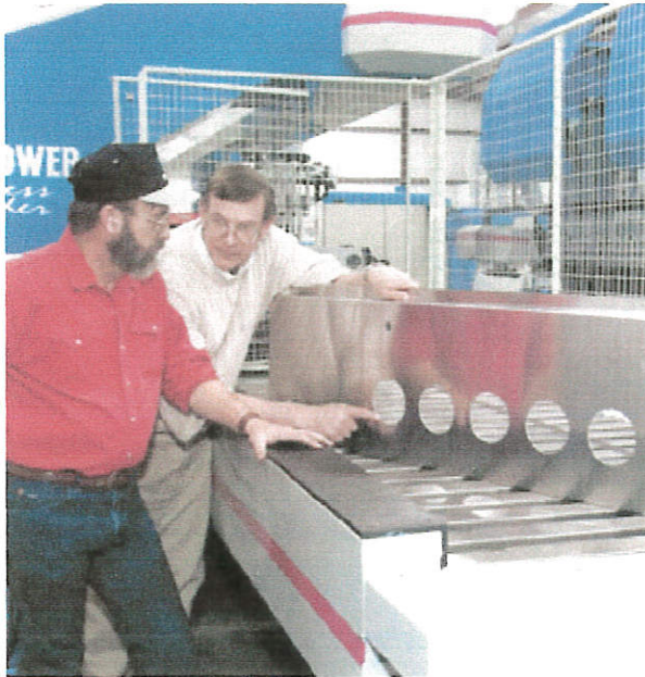
Bob McCann, assistant manager of metal fabrication, left, and Tim Gardner, vice president of manufacturing, check the results of their turret punch as the piece comes out of the folding machine. After automating, the company was able to shorten delivery time on some products by as much as five weeks.
