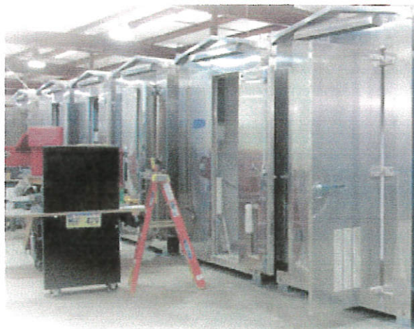
Signal equipment houses are nearly completed in production and await a shipping date in the PTMW fabrication facility in Topeka, Kan. Products are fabricated from aluminum, steel, stainless steel, and galvalume. Powder coating, bulletproofing, and wiring options are available.
