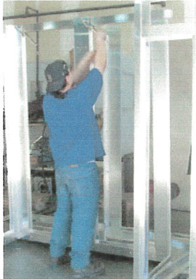
A worker clamps a vertical support in place before joining it with a weld. PTMW employs approximately 21 welders, who use GMAW and GTAW processes on aluminum, mild steel, and stainless parts.
