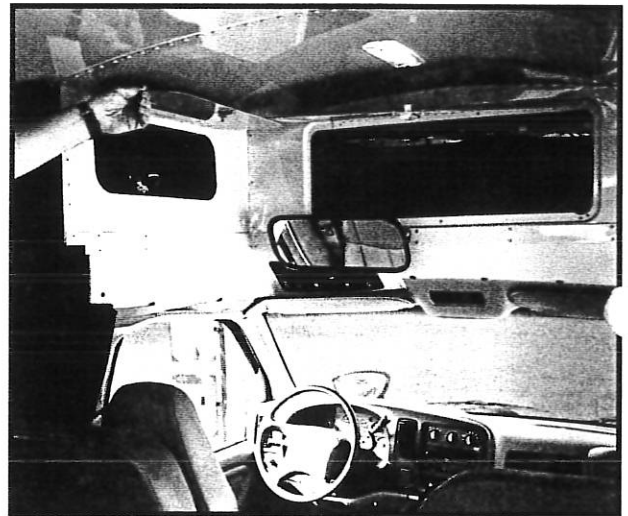
Electrical access and a convenient storage area are located in the driver's area.
