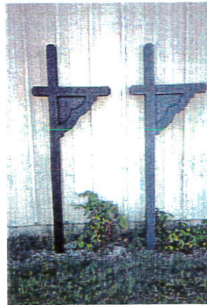
Mailbox posts manufactured from 50% wheat straw and 50% recycled plastic.
