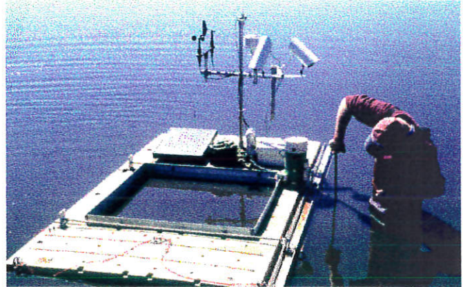
Below: A research assistant adjusts instrumentation to measure subsurface water temperatures.
