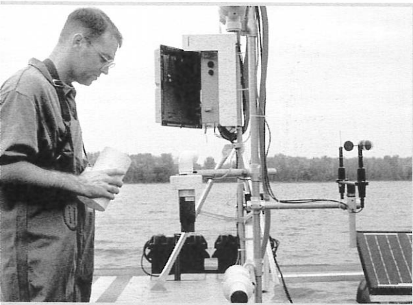
A device developed at K-State measures seepage in waste lagoons.
