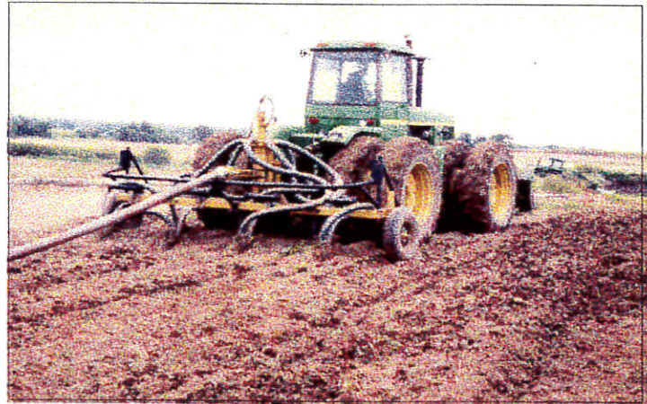
Above: Tractor applying liquid manure through a rubber hose to underground injectors.
