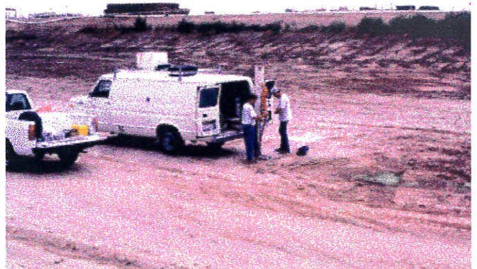
Right: Collecting soil cores from an 11-year-old lagoon using a direct-push soil probe. The lagoon had been dried and sludge removed prior to sampling.
