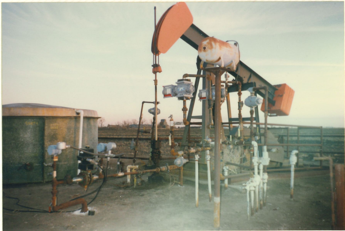
Irrigator takes ownership of gas at meter outlet at a price negotiated with gas well producer. 10,500 feet of irrigator owned gas lines move the gas to the 4 irrigation wells on this section (640 ac.)
