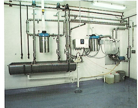
Milk from the parlor enters a De Laval Highline Receiver Group.
