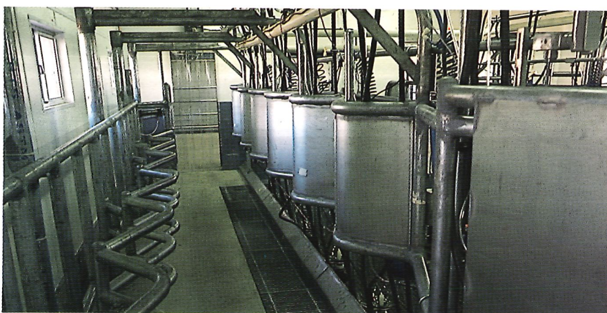
The self-indexing parlor stalls correctly position cows for milking. These stalls make movement of the cows smooth and efficient.
