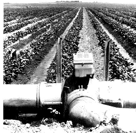
Surge flow system showing pipes carrying water, and a solar-powered control box, which is programmed to open the gates on an intermittent cycle. Chase County, Nebraska.
