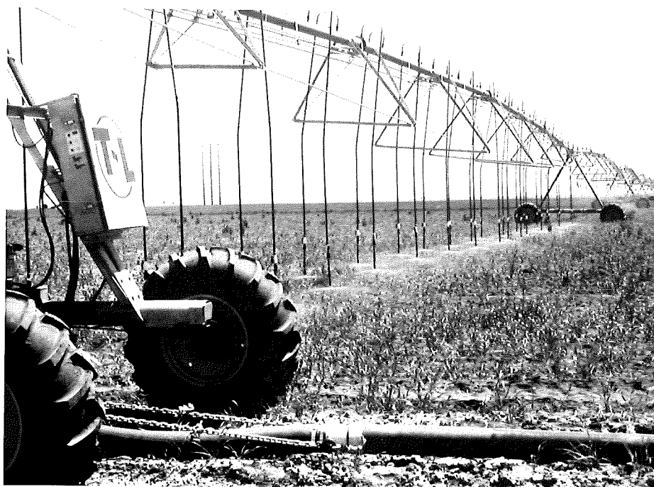
Drop tubes on a linear sprinkler system, at the Texas A&M research station, near Etter. The pipe in the foreground carries the water flow from the well and moves with the system. Moore County, Texas.
