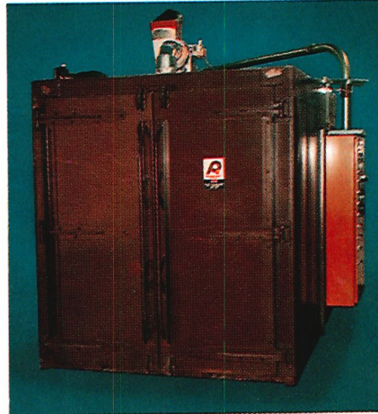
Our new oven provides baked-on enamel finishing and teflon coating baking.
