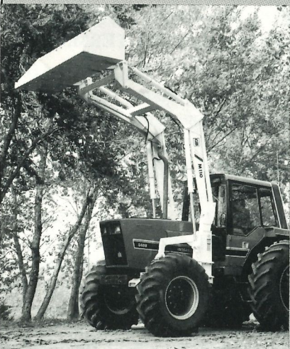
M 110 LOADER: with optional self-leveling. For 110 to 180 hp tractors.
