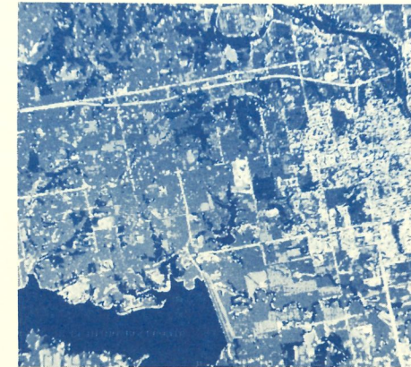
Land use/land cover map of Lawrence, Kansas and vicinity prepared by computer processing of Landsat 4 Thematic Mapper digital data.
