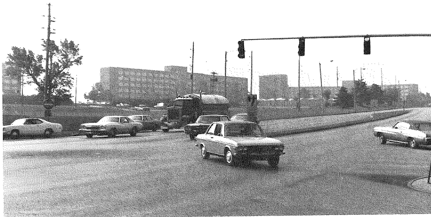
Careful synchronization of traffic signals can save significant amounts of fuel by reducing the amount of time vehicles spend waiting at red lights. The KU Transportation Center has provided assistance to Kansas communities in solving this complex traffic engineering problem.
