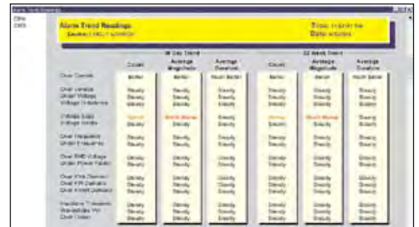
The circuit monitor's alarm trend log indicates whether alarm conditions are improving, holding steady, or becoming worse.
